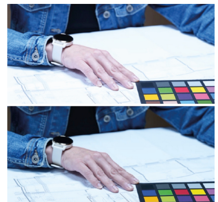
Figure 6: 6,000 K @ Planckian locus (top) versus 6,000 K BLL (bottom) with better contrast and richer color impression. © Lumitech. Real photographs; no image editing or AI used.
