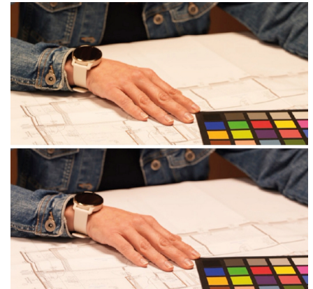
Figure 4: 3,000 K @ Planckian locus (top) versus 3,000 K BLL (bottom) with higher contrast and richer color impression. © Lumitech. Real photographs; no image editing or AI used.
