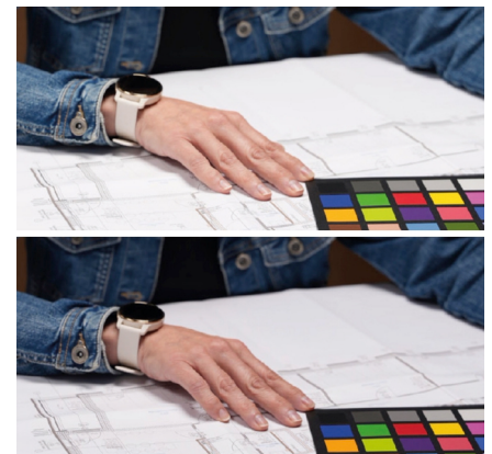
Figure 5: 4,000 K @ Planckian locus (top) versus 4,000 K BLL (bottom) with higher brilliance and richer color impression. © Lumitech. Real photographs; no image editing or AI used.
