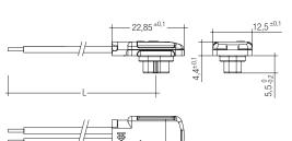
• Feeder cable for connecting a linear LED engine to a converter via QCS
