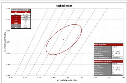
\*Data refers only to LED MODULES WITHOUT LENS! \*Colour shift through the lens is possible on request!
